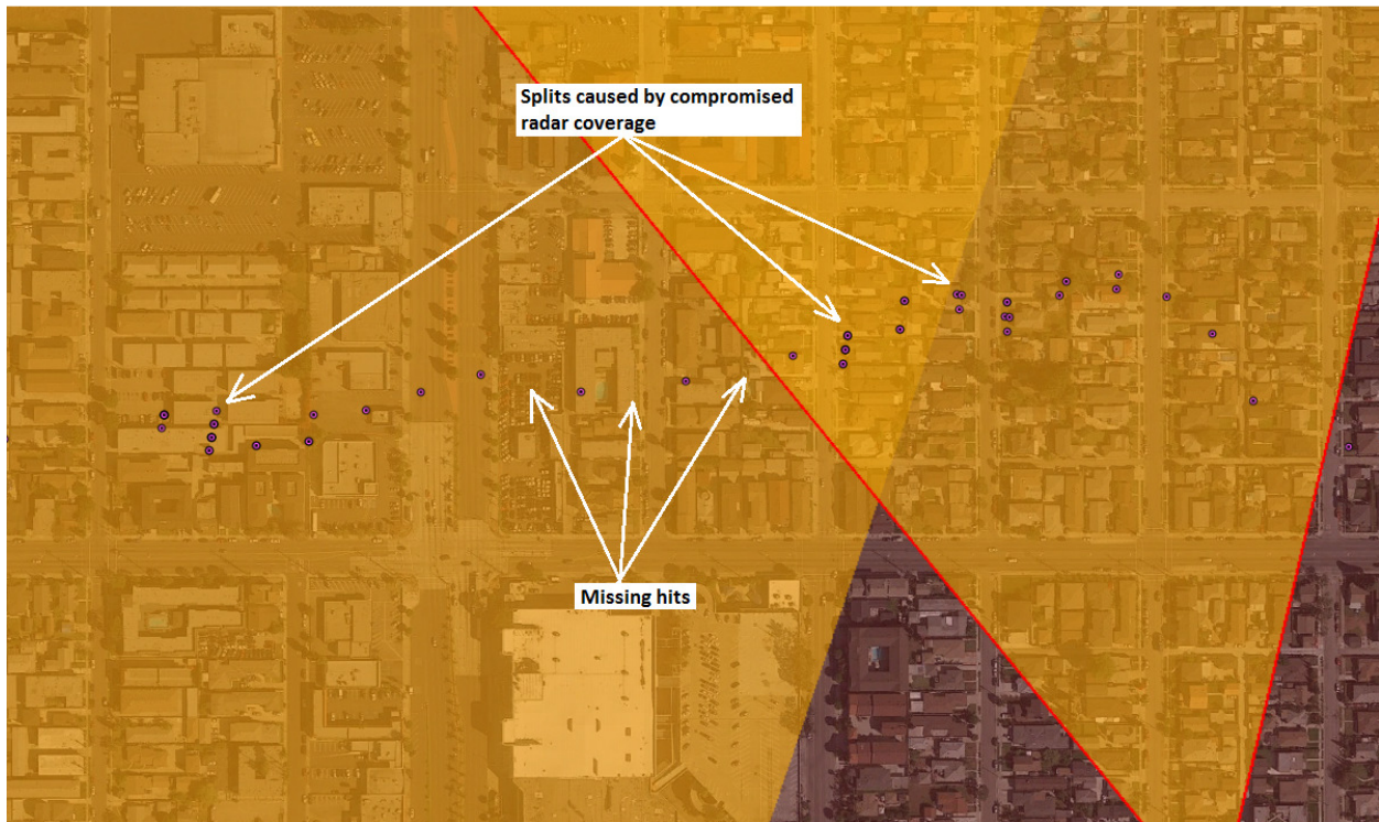
Figure 23 – Splits Indicating Compromised Radar Coverage
